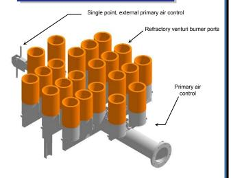
Multi-port burner with individual refractory burner ports shown. Other burner designs dependent on specific site gas heat energy densities
