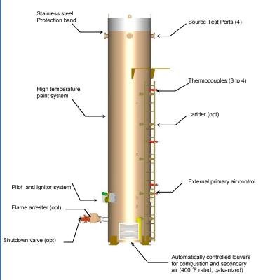
Flare must be operated with approved flame safeguard controls (optional)
